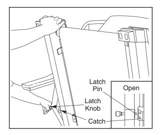
2. Hold the treadmill firmly with both hands, and lower the treadmill to the floor. To decrease the possibility of injury, bend your legs and keep your back straight.
